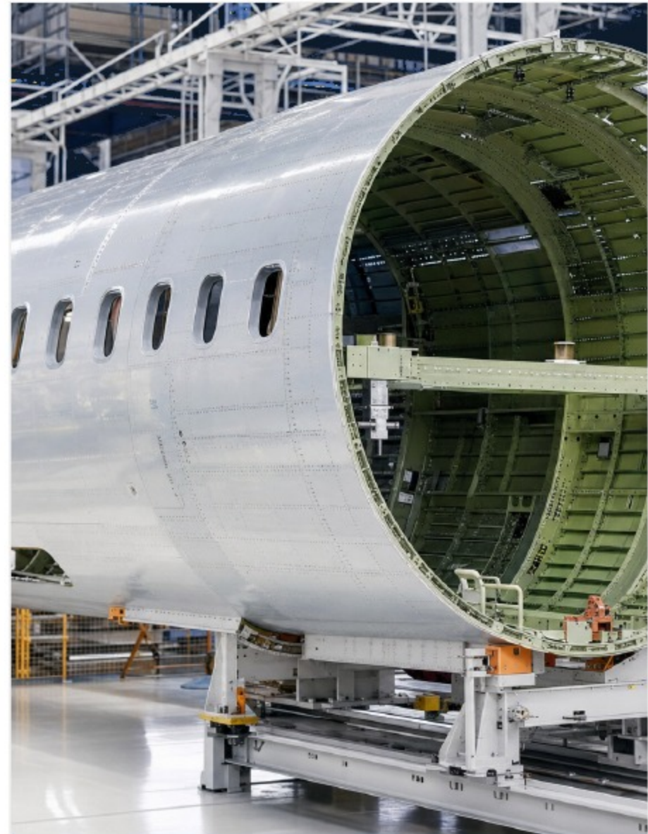
Aircraft fuselage construction — aluminum alloys enable lightweight aerospace structures
